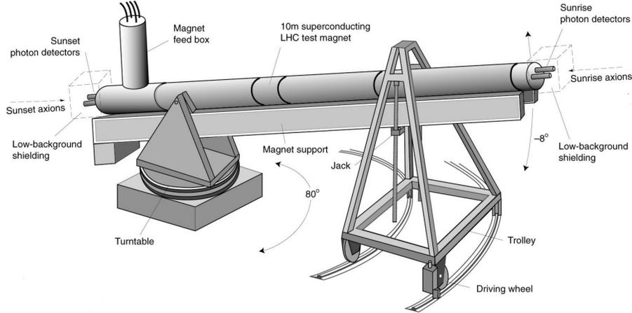
Figure 2. Schematic view of the CAST experimental setup. The 10 m long LHC prototype magnet can move  $\pm 8^\circ$  vertically and  $\pm 40^\circ$  horizontally.
