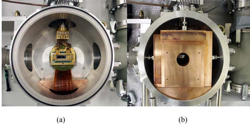
**FIGURE 1.** (a): The pn-CCD detector with its vacuum housing. The pn-CCD chip is the central black part surrounded by a gold plated cooling mask inside of the aluminum vessel. (b): The same picture with the internal passive copper lead shield being installed. The circular hole in the shield provides the aperture towards the X-ray optics.
