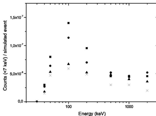
**FIGURE 3.** Simulated response of the CCD detector to the external gamma background: events in the region up to 7 keV per simulated photon as a function of the energy of the incident photons. Four shielding conditions have been considered: with no shield (squares), with the internal copper shield (circles), with the internal copper + external lead shields (triangles) and with internal copper + external lead + internal lead shields.
