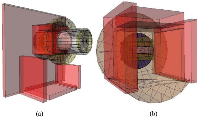
**FIGURE 2.** (a): View of all simulated components, including shield, aluminum vessel and connection to telescope. (b): View of simulated components inside the aluminum vessel, including copper and lead shields and detector.
